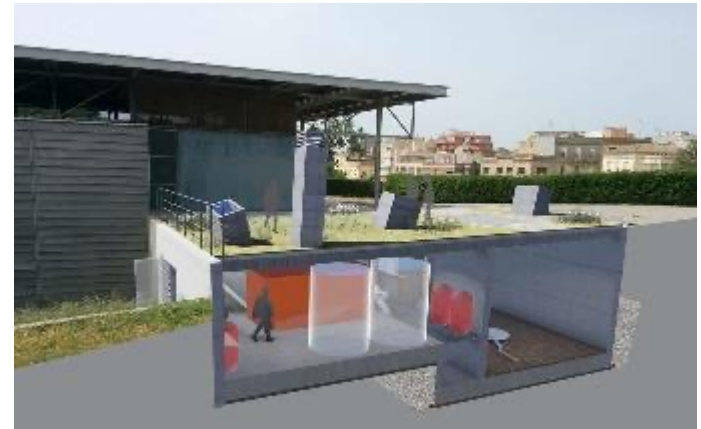
“La Girada” (Vilafranca del Penedès, Spain): 500 kW boiler fueled with vineyard prunings for municipal district heating. Image source: Vineyards4heat project
