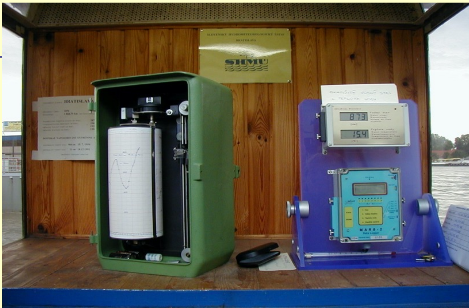
MARS 2 – Automatic registration device with pressure sensor
