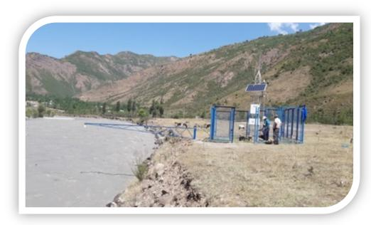
On the rivers, observations are made of the level, discharge, water temperature, precipitation and ice phenomena.
